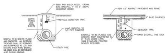
UTILITY LINE INSTALLATION (UNPAVED AREAS) N.T.S.
